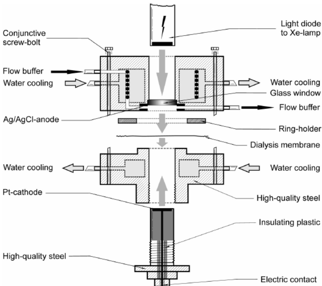
Figure 2.1: The interior structure of the home-built Joliot electrode [16, 18]
